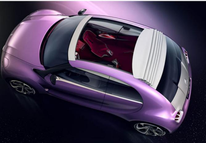
REVOLTE JE PLUG-IN HYBRID, BATERIE, KTERÉ NAŠLÝ MÍSTO V ZADNÍCH SEDADELECH, JE TĚDY MOŽNÉ DOBLUET Z BĚŽNÉ ELEKTRICKÉ ZÁSUVKY. AUTOMOBIL JE TAKÉ SCHOPEN JIZDY CÍSTĚ NA ELEKTRINU. NA SHRNOCOVACÍ STŘEŠE JSOU UMÍSTĚNY SOLARNÍ PANELY, KTERÉ SE STARAJÍ O NAPÁJEJENÍ PALUBNÍCH SYSTÉMU.
